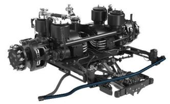
The Texelis manufactured bogie system fitted to the Siemens Neoval APM.
